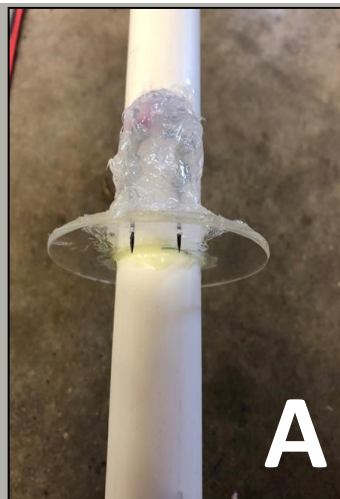
Figure 2. Gradient probe used to measure field intensity at 0.457 m, 0.914 m, and 1.372 m below the water surface: (A) gradient probe points spaced 1 cm apart to collect field intensity at each depth; (B) floating disc attached to gradient probe and three leads for oscilloscope attachment; (C) floating gradient probe with rubber hose attached to extendable pole used to rotate the probe at each sampling location while standing in the boat.
