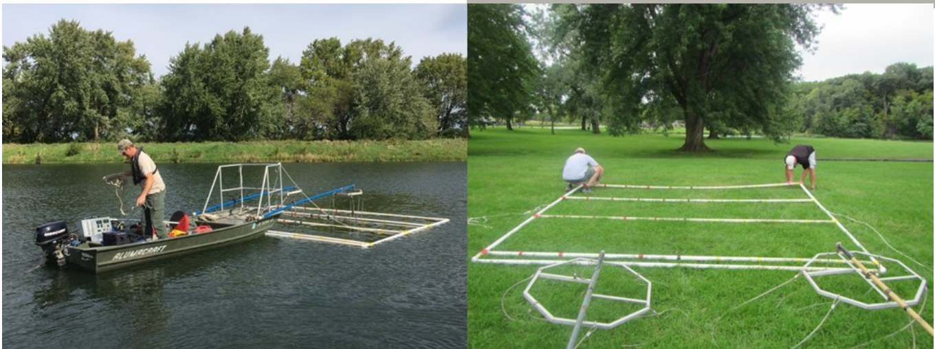
Figure 1. Sampling grid used to guide collection of 132 electrofishing field intensity points.
