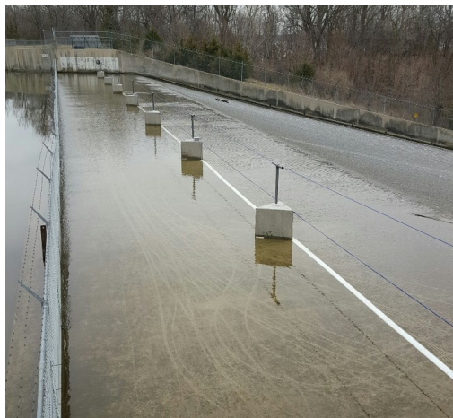
PIT tag antenna installed on the outlet of Big Creek Lake.
